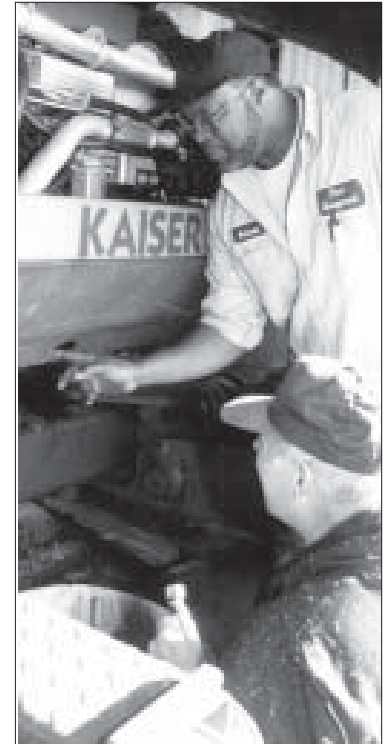
Fleet Management Director Fred Claussen, right, briefs Chris Moreda, director for the day. Right: Mechanic Johnny Armwood shows Claussen where to attach the hose to drain the oil from the excavator.
